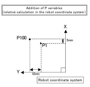
An example of relative calculation(Addition) 10 P2=(5,10,0,0,0,0)(0,0) 20 <u>P100=P1+P2</u> 30 MOV P1 40 MVS P100 P1=(200,150,100,0,0,45)(4,0)
