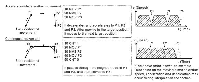
Fig.4-7:Acceleration/deceleration movement and continuous movement
