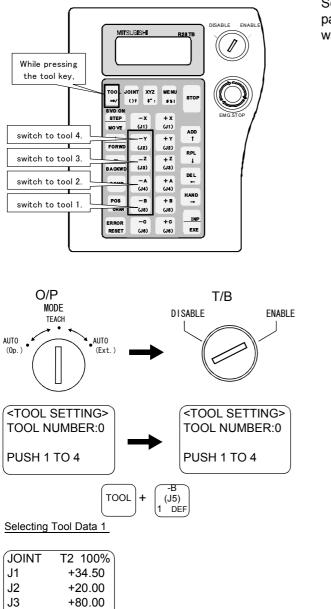
Set the tool data you want to use in the MEXTL1 to 4 parameters, and select the number of the tool you want to use according to the following operation.
