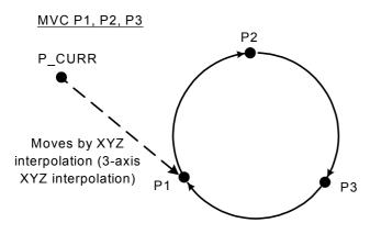
Fig.4-11:Example of circle interpolation motion path
