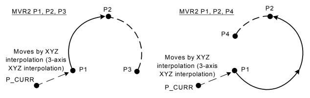
Fig.4-13:Example of circular interpolation motion path 2
