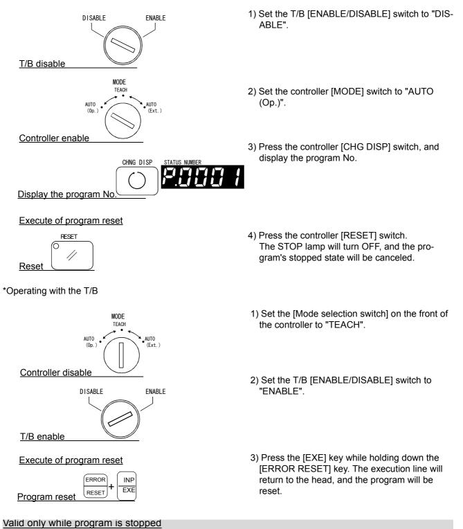
The program cannot be reset while the program is running. Always carry out this step while the program is stopped.
