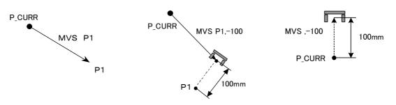
Fig.4-15:Example of movement at linear interpolation
