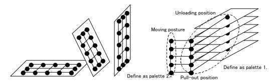
The pallet instruction can define lattices as shown in the illustration above. This makes it possible, for example, to easily create coordinates such as the holding position and front position of works arranged in layers. Of course, it is possible to calculate these positions without using the pallet instruction, but using the pallet instruction can reduce the cycle time since calculations can be performed with a single instruction.
