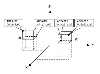
When operation is performed together with peripheral devices, work area may have to be shared. Under such circumstances, one device must let the other know when it is within the shared area. For this purpose, a robot can be configured to output a signal while it is in a certain area by setting parameters.
