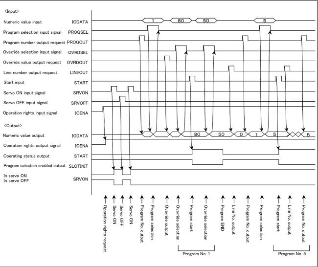
Fig.6-3:Example of external operation timing chart (Part 2)
