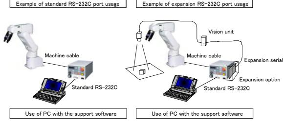
Caution)The example above is for robot controller CR1. Controllers other than the CR1 do not require expansion option box.
