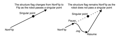
(8) If the singular point passage function is specified, the operation speed may be lowered compared to normal linear interpolation, etc. Moreover, the singular point passage function may affect the execution speed of programs as the function involves complicated processing. Specify the singular point passage function only for interpolation instructions where the function is required.
