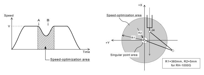
Fig.4-20:The situation of the speed at speed-optimization.
