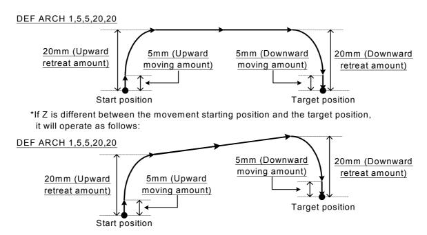
Fig.4-10:Example of arch interpolation motion path (seen from the side)
