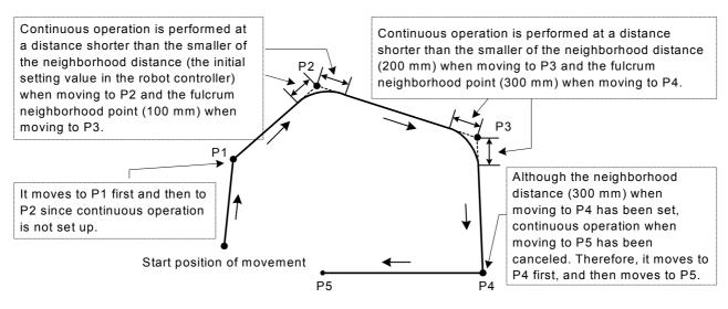
Fig.4-6:Example of continuous path operation
