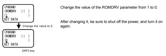
(7) Switching to the high-speed RAM operation(DRAM operation)
