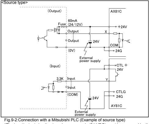
\*The input/output circuit external power supply (24 VDC) must be prepared by the customer.
