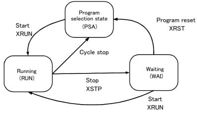
Fig.4-2:Operation state of each slot
