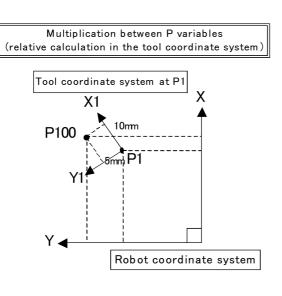
An example of relative calculation (multiplication) 10 P2=(10,5,0,0,0)(0,0) 20 <u>P100=P1\*P2</u> 30 MOV P1 40 MVS P100 P1=(200,150,100,0,0,45)(4,0)
