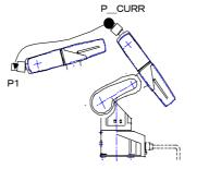
Fig.4-9:Example of joint interpolation motion path
