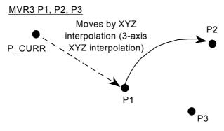
Fig.4-14:Example of circular interpolation motion path 3
