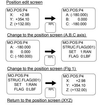
1) When the position edit screen is displayed, the coordinate values of the X, Y, and Z axes are displayed first. Press the [RPL] key to display the data of the A, B, and C axes.
