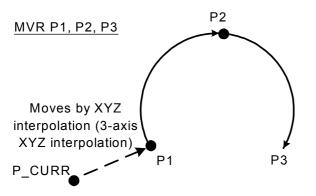
Fig.4-12:Example of circular interpolation motion path 1
