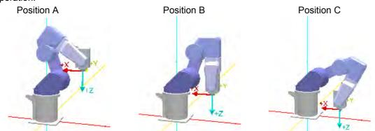
The robot can pass a singular point when the robot's motion path passes through the singular point. If the motion path does not go through the singular point (passes near the singular point), the robot continues operation without switching the value of the structure flag.
