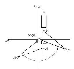
Fig.4-19:When passing through near the origin point by linear interpolation
