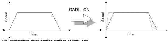
Fig.4-18:Acceleration/deceleration pattern at light load
