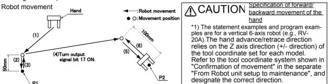
' Moves to P1 with 3-axis orthogonal interpolation.
