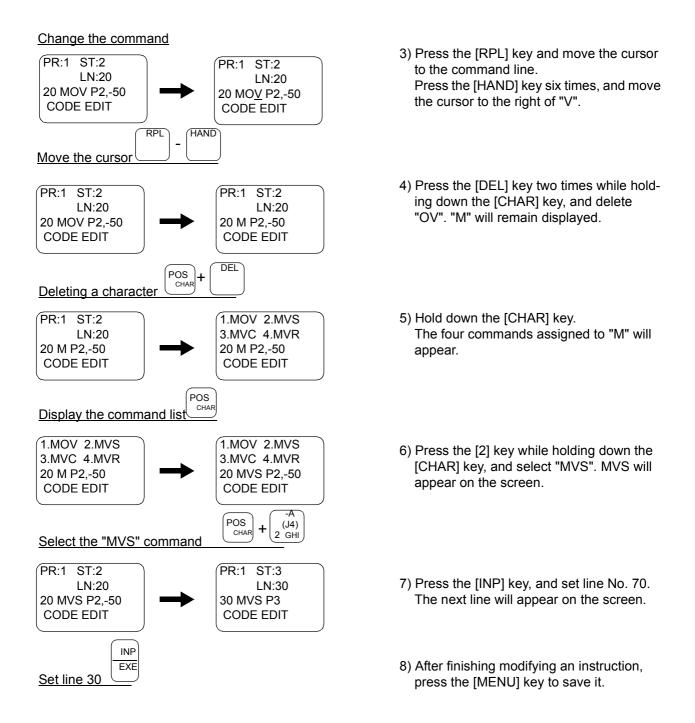
Line No. 20 has been changed to linear movement with the above operation.
