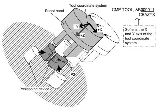
Fig.4-5: The example of using the compliance mode
