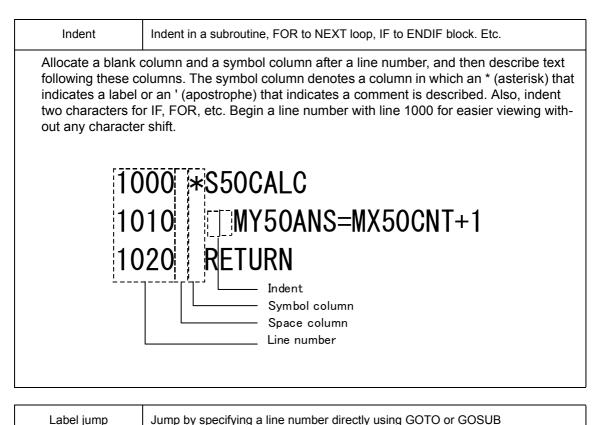
Line number jump is prohibited as it will interfere with the visibility of programs. Be sure to jump by providing labels.
