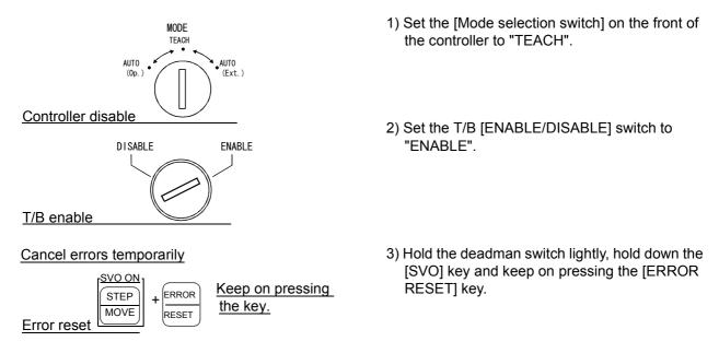
The operation above will reset errors temporarily. Do not release the key; if it is released the error occurs again. Perform a jog operation as well while keeping the [ERROR RESET] key pressed.
