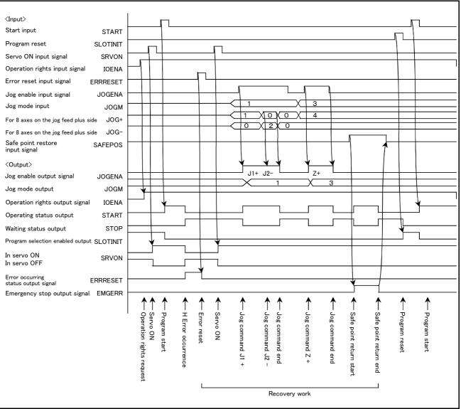
Fig.6-5:Example of external operation timing chart (Part 4)
