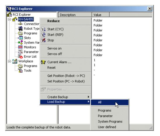
Select the folder that contains your backup data. After your data is successfully recovered, switch the robot controller off and back on again to confirm the changes.
