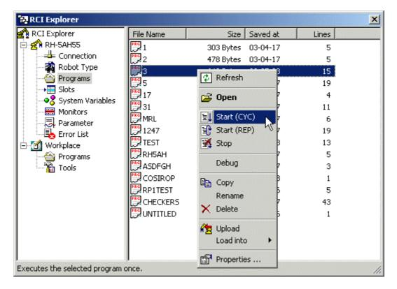
There are two commands to start a robot program. Use the command "Start (CYC)" (1 cycle) to start the program, once. Use the command "Start (REP)" (repeated) to start the program in a continuous loop. With the command "Start (REP)" the program continues until the program is stopped by a user command.
